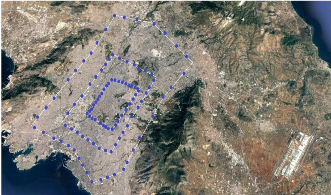
Image 11: Hypothetical cycles created on Google Earth (Blue dots-Places of the bins, White rows-Routes of collection).
